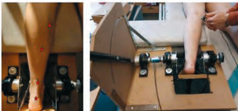
Figure 1 : Anatomical points tested and biomechanical setup for stiffness
